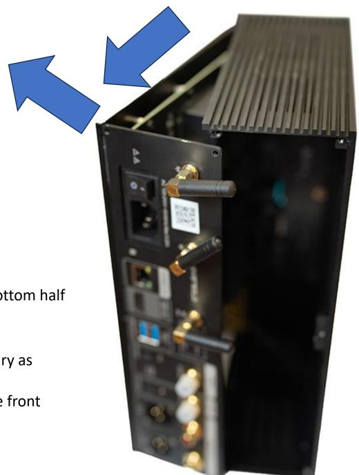
Step 3: Holding the top cover firmly, pull the bottom half slightly backwards and to the side.
