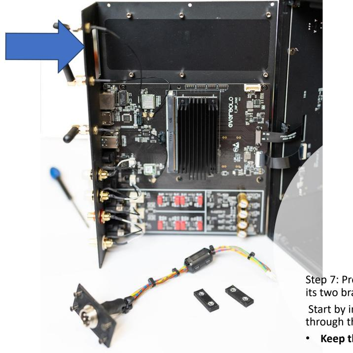
Step 7: Prepare the panel adapter and its two bracings.
