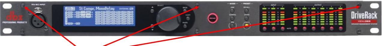
Remove top screws using Allen key (or Torx #20)
