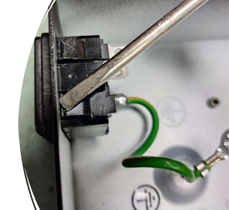
• Step 4: Repeat step 3 at the bottom side, remove the power entry socket.
