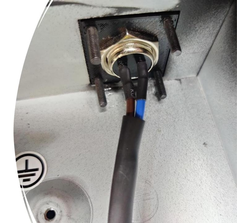
• Step 8: place the panel adapter fasteners, place the 3mm bolts. Note: do not over-tighten the screws!
